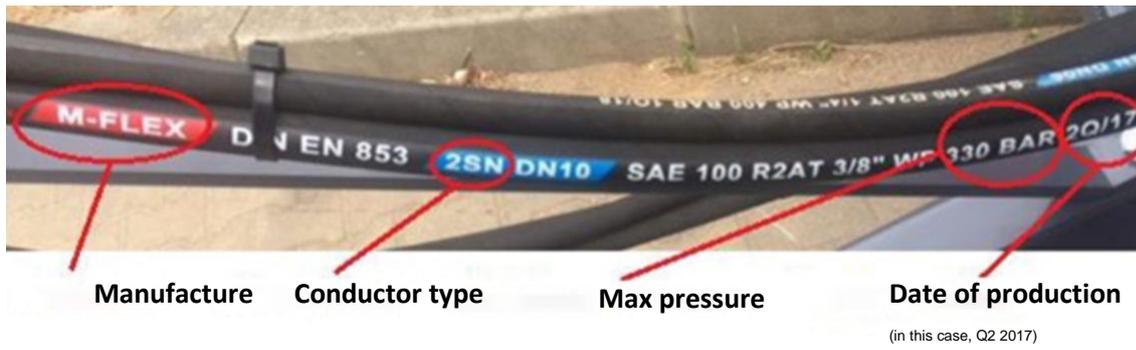
**Figure 25.** Marking of the hydraulic lines
