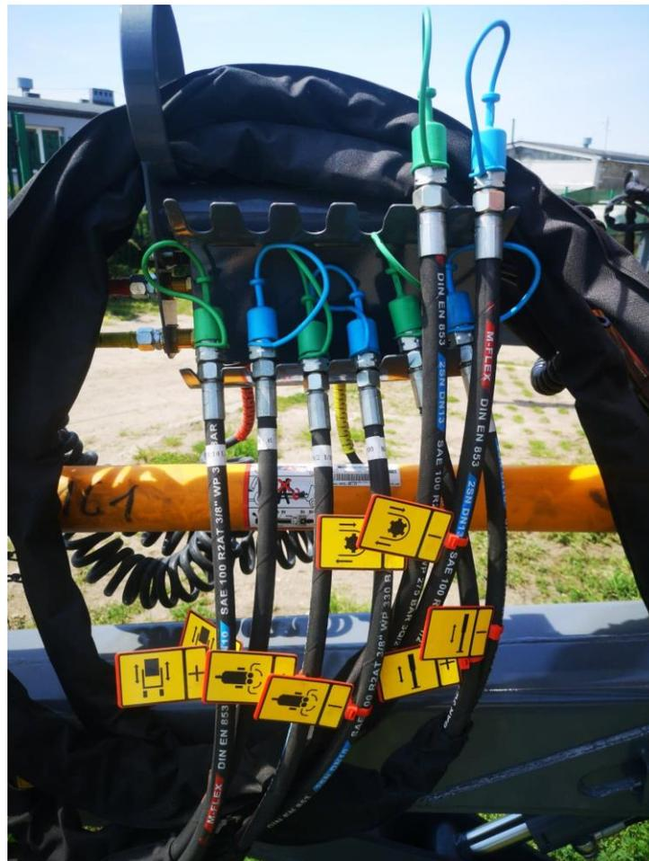
**Figure 26.** Pictograms on the hydraulic connectors for easier connection to the tractor (standard)
